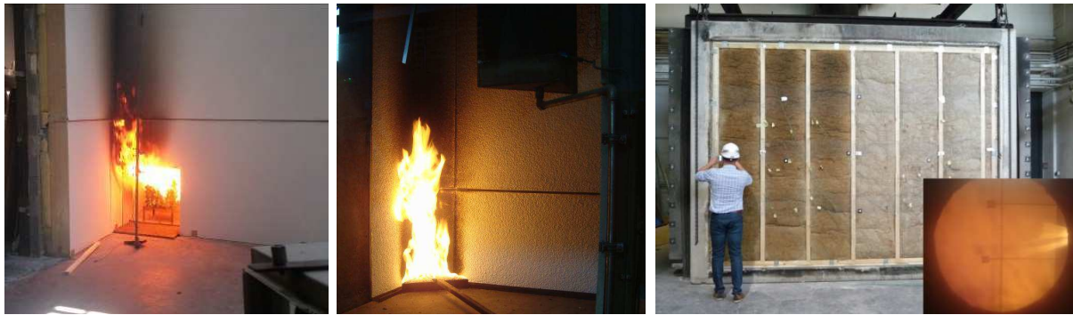
FIGURE 2-11: FIRE BEHAVIOUR AND FIRE RESISTANCE TESTS TO PROOF THE FIRE SAFETY OF PREFABRICATED FACADE ELEMENTS [4, 5]
