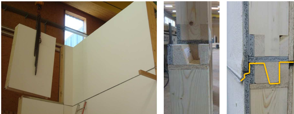
FIGURE 2-10: SAMPLE OF THE E.T. FAÇADE SYSTEM (LEFT) AND A HORIZONTAL JOINT DETAIL (RIGHT) [4]
